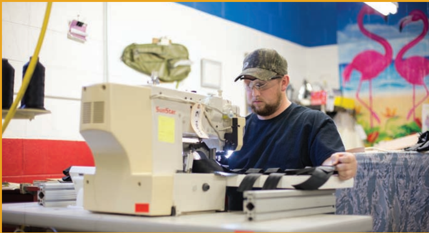
Brad Pierce, machine mechanic of Four Rivers, sews a webdoor for the postal service on one of the new pattern trackers. The webdoor adheres to both ends of a cart that USPS workers use to move mail.
